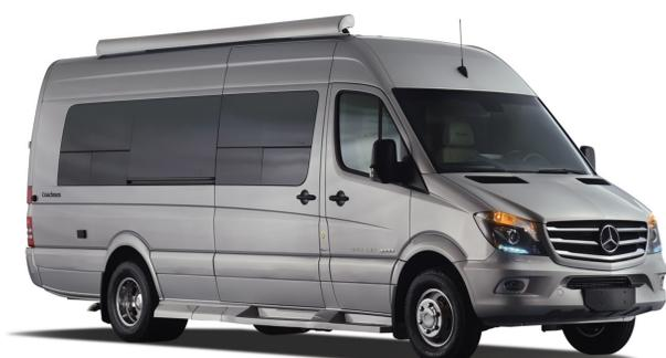
In a compact RV application, a comprehensive inverter system may be easier to package than an on-board generator. The Coachmen Galleria is just one example of a small motorhome that uses inverter/charger and battery power exclusively.
