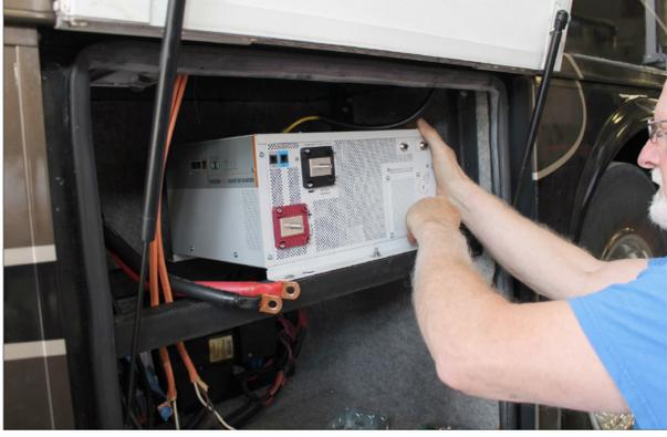
The Freedom SW features premium sine wave output with high surge capability and temperature compensated, power-factor corrected, multi-stage charging to meet power needs of demanding loads including inductive motor loads. Available in two 24-volt DC models (which requires special wiring, and comes as an option in some new Class B motorhomes), the Freedom SW offers series and parallel stacking capability to enable twice the rated output and operation of 240-volt AC applications, respectively.
