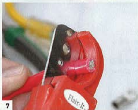
[4] Once the wires and connectors are contained, the strain relief is put in place and the cover [5] is reinstalled for a clean look. [6] A 50-amp (specified by the manufacturer) marine-grade circuit breaker was used to protect the charger. [7] Insulation on the 4-gauge marine-grade electrical cable is stripped to get ready to install the terminals.
