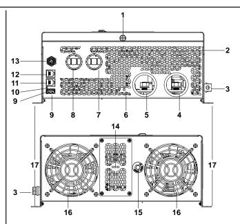
Figure 3 AC/DC and GFCI Panel for Marine Models
