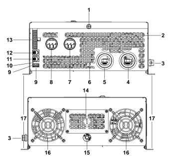
Figure 2 AC/DC and GFCI Panel for Standard Models
