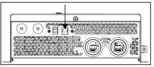
**NOTE**: When the remote panel is connected, turn the inverter/charger's Power button to to Standby (up position). This allows the remote panel to control the inverter/charger's power status.
